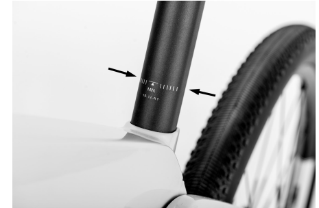
Figure 39: Seat post (maximum extension length).
