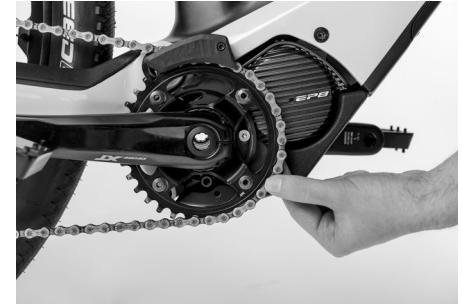
Figure 22: Checking the condition of the chain
