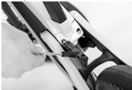
Figure 40: Clamping screws/AERO seat post
