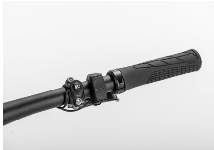
Figure 24: The position of the shifting lever (electronic)
