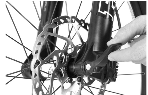
Figure 53: Fitting the Cross front wheel axle system
